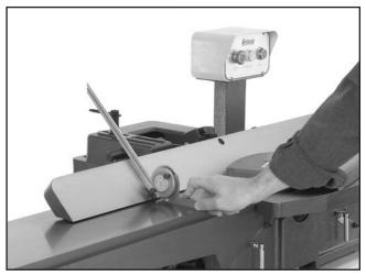
Figure 51. Adjusting fence 45° outward.
